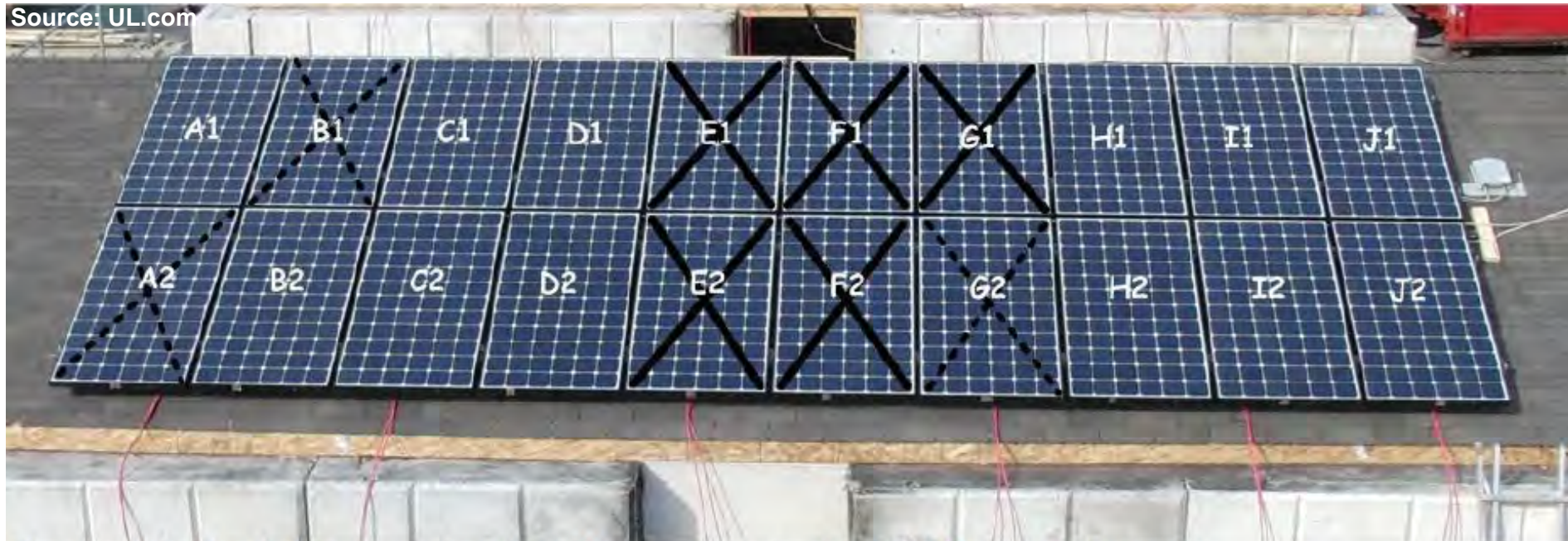
Figure 112 Roof diagram after fire: X = no power, dashed-X = partial power
