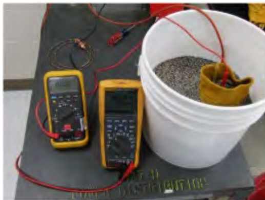
Figure 29 Testing a glove in metal shot
