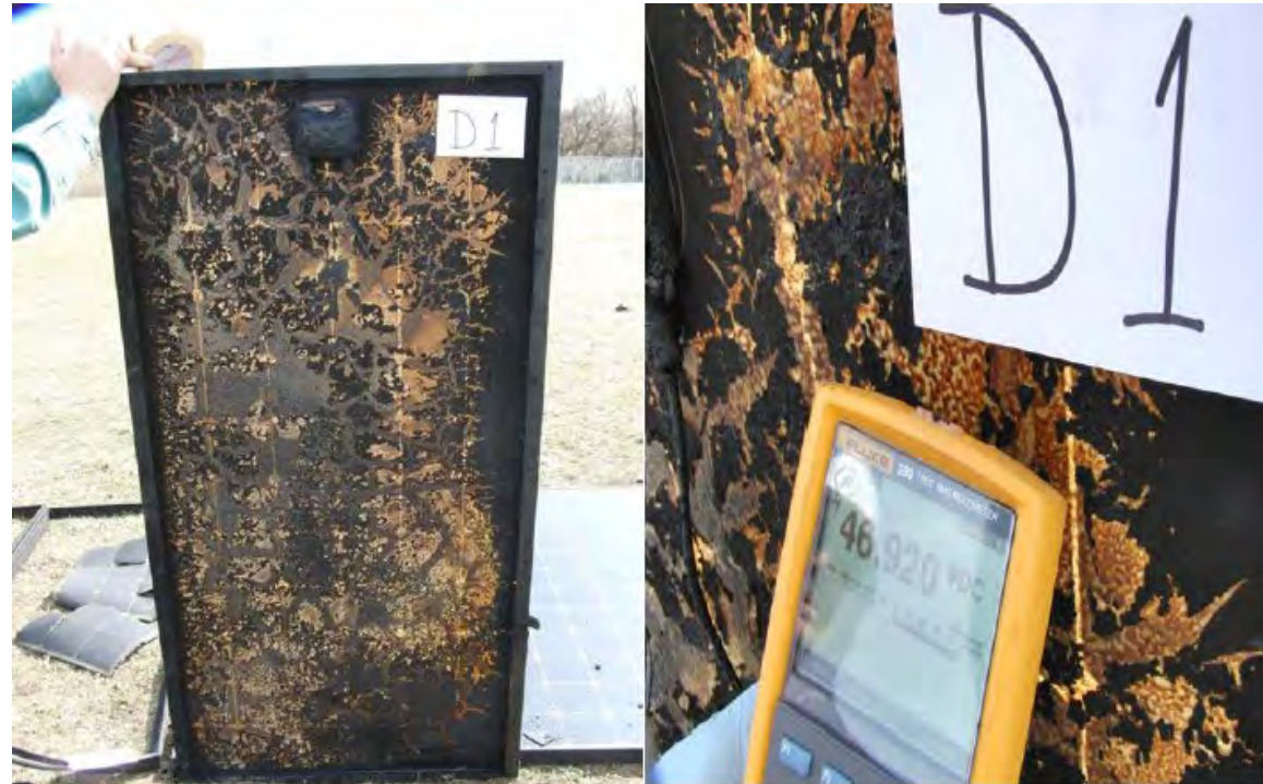
Figure 117 - Module D1 – badly burnt on backside, but functional and producing full voltage
