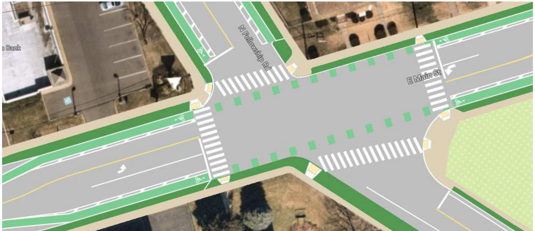
Figure 80: Concept design, Main Street at Fellowship Road Source: DVRPC, 2023, created using Remix
