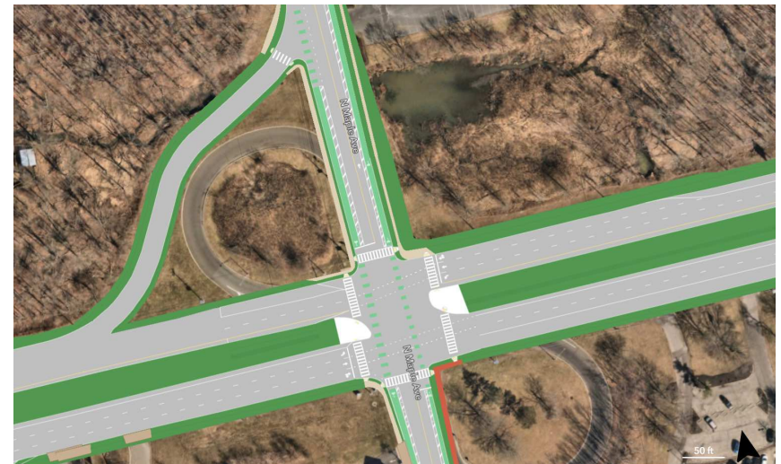
Figure 47: Proposed road diet and jughandle closure at Rt. 70 and N. Maple Ave.
