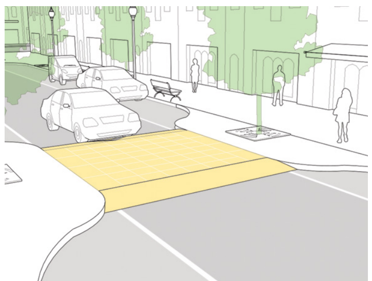
Figure 50 Example diagram of a speed table
