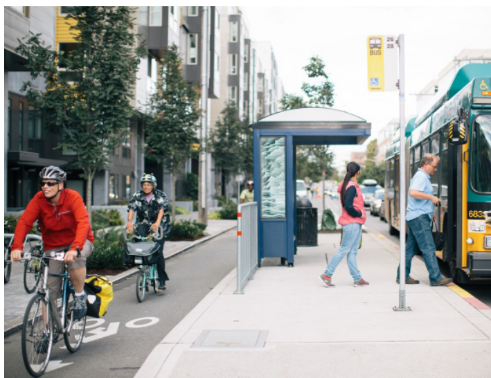
Bus bulbout with rear bicycle lane
