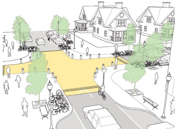
Figure 58 Raised intersection diagram
