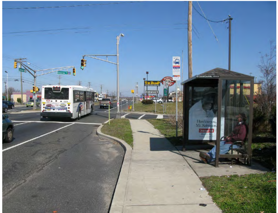
Bus stop with no pedestrian facilities along NJ 42 in Turnersville (pictured left) was improved with sidewalk connections, bus stop pull off, and bus shelter (pictured above).
