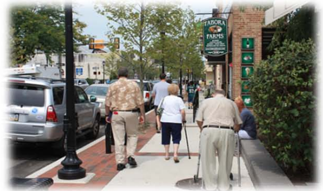
New streetscape enhancements have been installed along Main Street from Broad to Richardson and a small portion of Broad Street. Enhancements include new brick pavers, curbs, parking meters, light posts and parking space delineation. The streetscape improvements are part of the borough’s $2.3 million revitalization effort to bring visitors and residents to the downtown.
