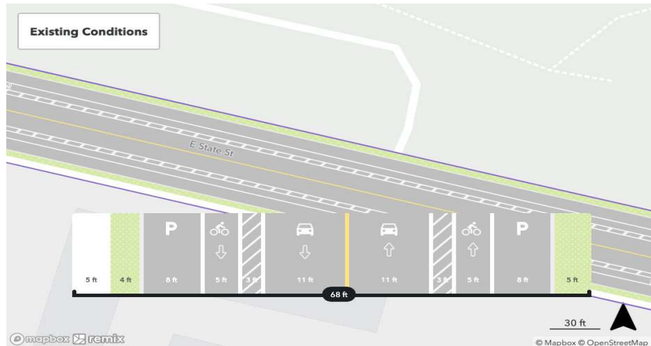
Figure 8: E. State Street Existing Conditions
