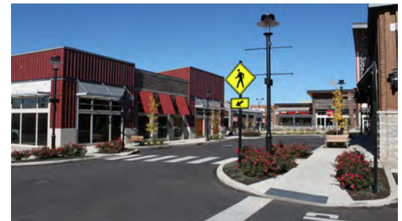
The KOP Town Center combines a variety of elements, such as building design, continental crosswalks, signage, and curb extensions, to prioritize pedestrian mobility.
