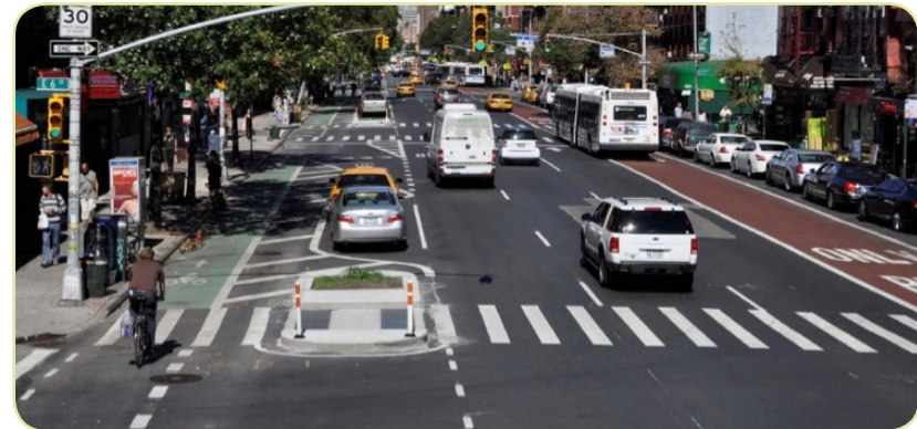
FIGURE 19: Example protected bicycle lane with pedestrian islands
