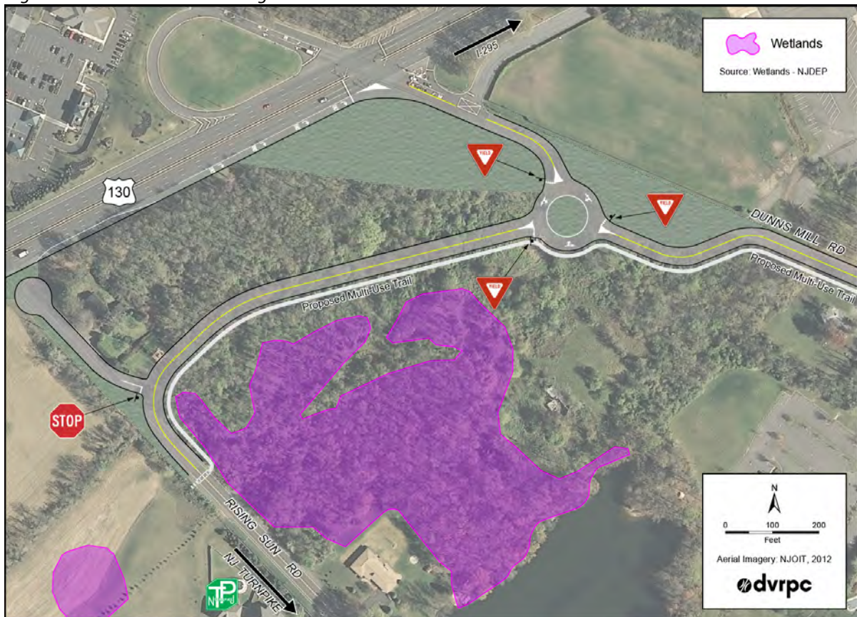
Figure 9: New Connector Road Alignment
