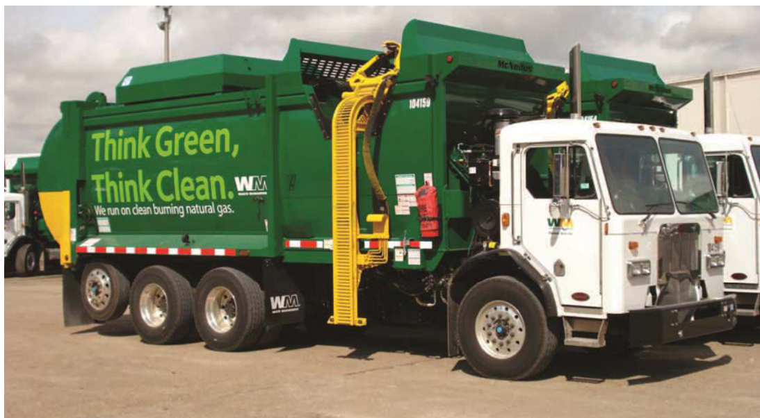
Figure 21. Waste Management's compressed natural gas refuse truck
