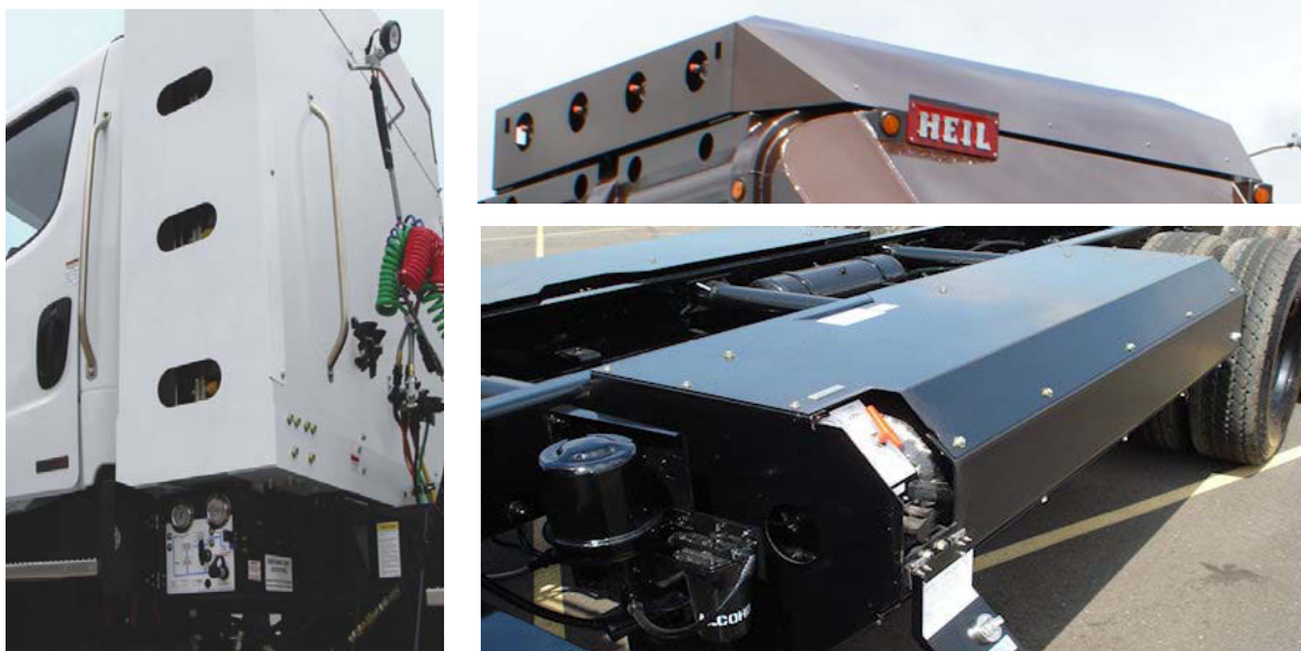
Figure 9. Compressed natural gas vehicle storage tank configurations: behind the cab, on the roof, or within the chassis
