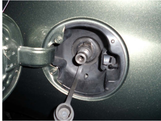
Figure 6. P36 CT1000 compressed natural gas receptacle
