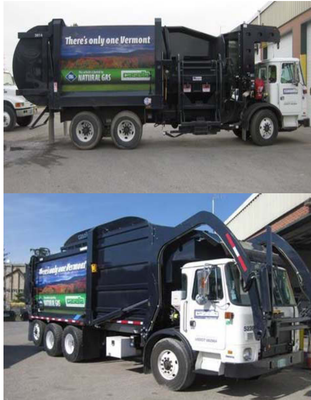
Figure 19. Autocar dedicated CNG refuse trucks with Cummins-Westport ISL G CNG engines in front and side-loader configurations.
