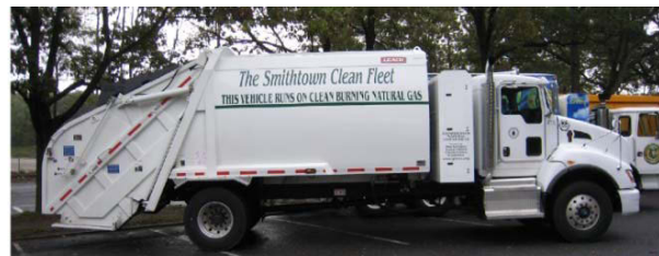
Figure 23. Smithtown 2010 Kenworth T440 CNG refuse truck with pedestal mount fuel system
