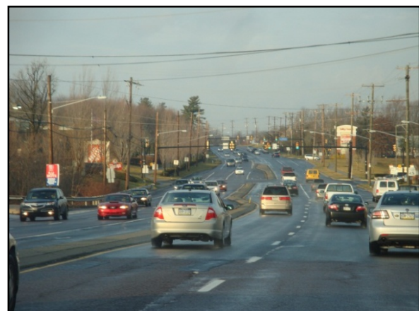
Figure 6: Center Median and Auxiliary Turning Lanes
