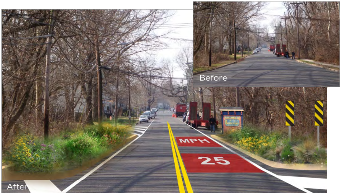
Figure 21: Simulation of Traffic-Calming Recommendations along Elizabeth Street
