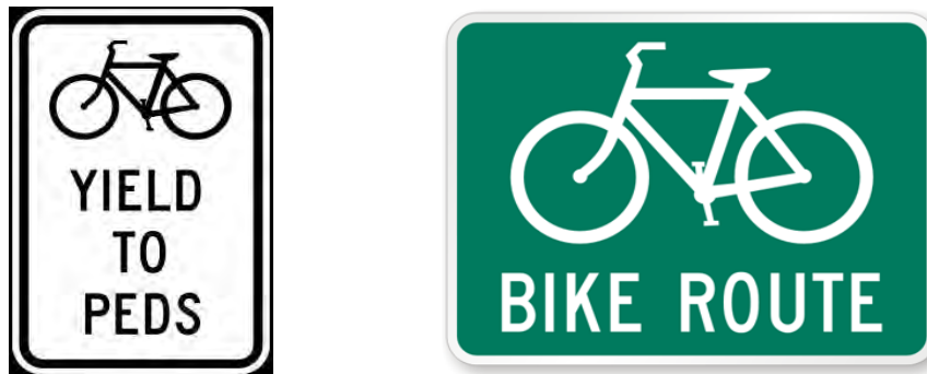
Figure 4: Example MUTCD bicycle facility signs
