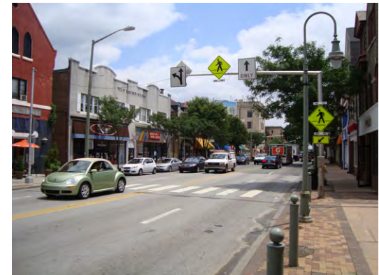
The lane control signage detracts from the pedestrian warning signage.
