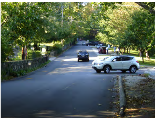
Adding edge lines will visually narrow the wide roadway and delineate the parking area at the playground.
