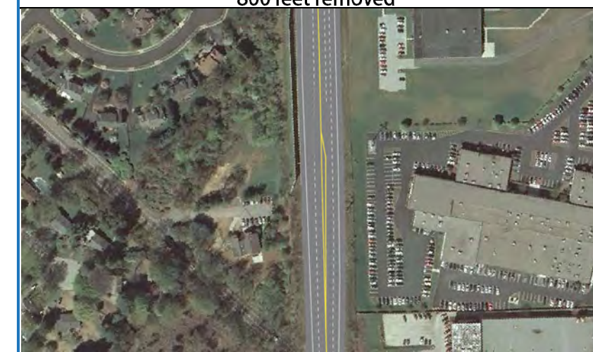
Concept of the westbound I-76 transition (one-quarter mile), favoring heavier US 202 / US 422 collector-distributor roadway volume versus the express lanes to the Turnpike. (DVRPC)
