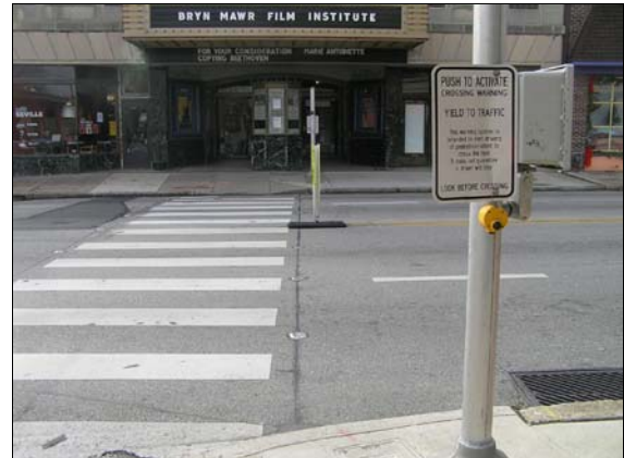
Well-marked crosswalk over Lancaster Ave. south of the station with in-street pedestrian yield sign.
