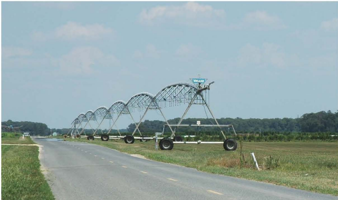
A center pivot irrigation rig - a type of overhead irrigation.
