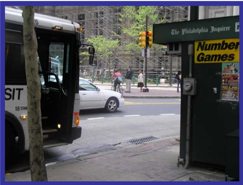
Newspaper stand blocks sight distance at Juniper Street
