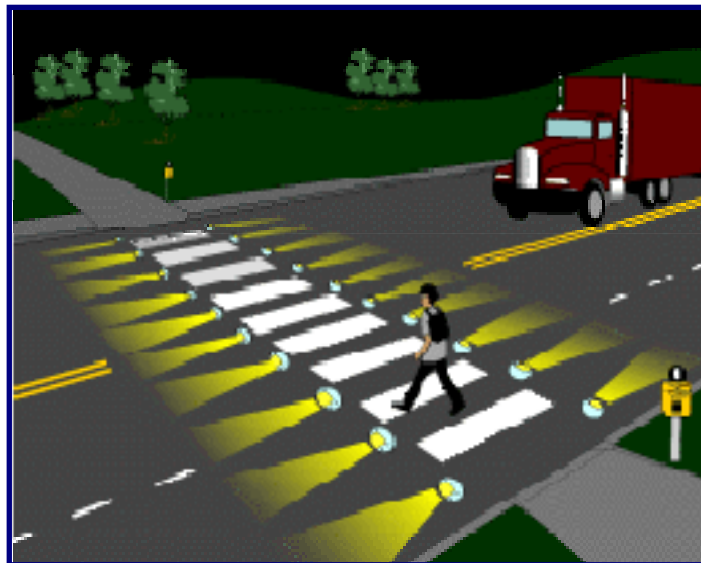
Figure 3: In-pavement Lighting at Crosswalk
