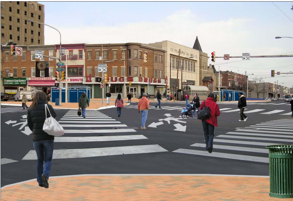
Top: Current appearance of the Broad/Erie/Germantown intersection; Bottom: Conceptual illustration of a pedestrian scramble treatment at the intersection, along with other minor aesthetic improvements (including the removal of billboards)
