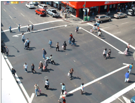
Example of two-street scramble in Oakland, California (Source: Traffic Safety Center, University of California at Berkeley).
