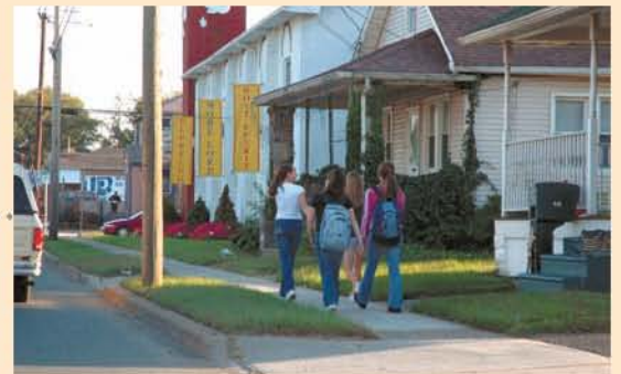
A Strip of Green. The grass verge creates a comfortable separation between cars and pedestrians.
