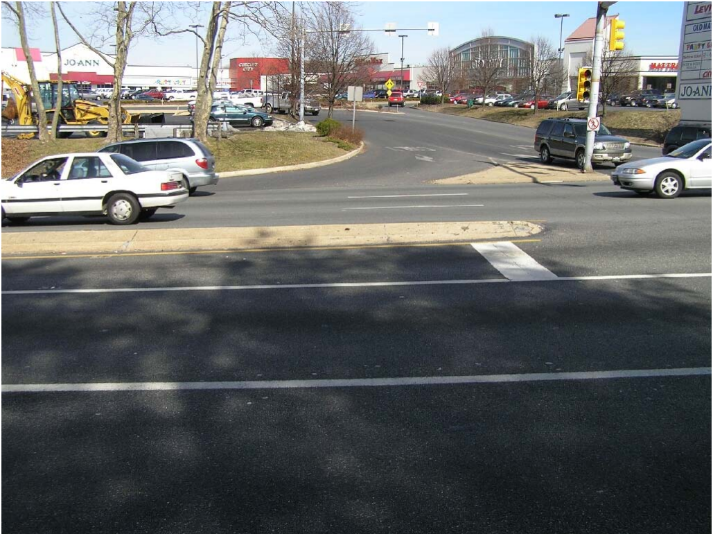
Marple Shopping Center EB, existing right turn lane “yield” movement proposed to be made a “signal controlled, NO TURN ON RED” movement
