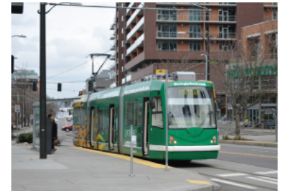
Figure 57 | Curb extension, Seattle Streetcar Source: Eric Strathmire via Flickr (CC BY-NC-ND 2.0)
