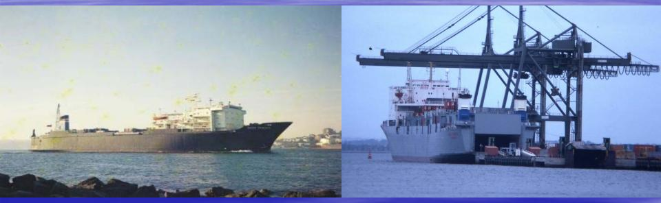
ANL's Bass Trader Built1976 GRT : 6,374 NRT: 2,170 net. DWT: 7,483 dwt. Lbd: 141.97 x 23.42 x 7.182m Vehicles under deck Containers on deck Bow Thruster + Twin screw – CPP Service speed 14.5 knots.
